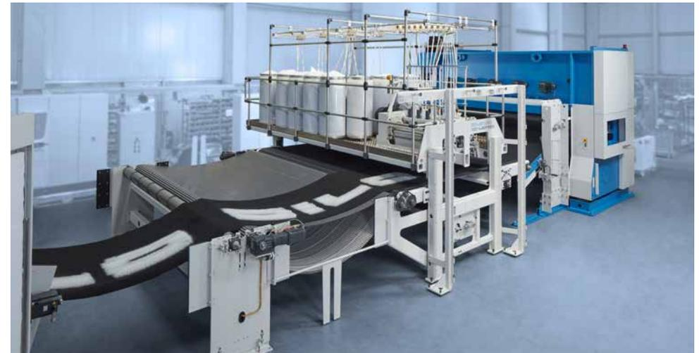
*“Additive textile manufacturing” with 3D-Lofter and DI-LOOM OD-II SLC HαV 35*
