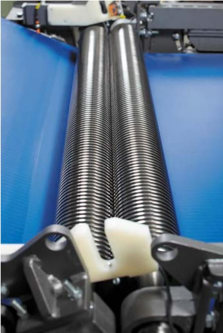
CV1-System – Pre-compensation of thick edges to get an even cross profile
