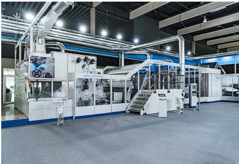
The revised HyperLayer NT for the presentation of the latest state-of-the-art highspeed precision layering technique showed new standards, which play an important role especially in hydroentanglement lines. In this application, it is important to achieve layering speeds up to 190 m/minute using sophisticated viscose fibres and a layering width of about 4 m while at the same time showing high layering precision in cross and longitudinal direction.
